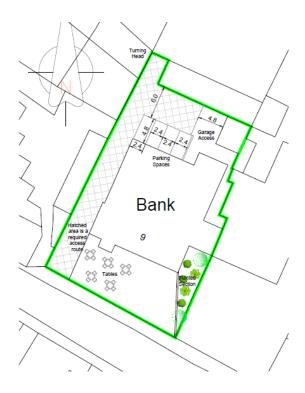
Access for staff and deliveries is taken from the SW of the site which is shown as hatched on the above plan. The area to the front of the building is proposed to be used for outside seating with a section to the SE proposed to be planted.
